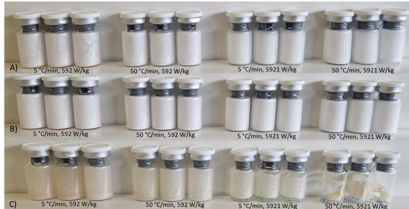
A) trehalose, B) mannitol, and C) sucrose-mannitol samples after 13 weeks at 50 °C
