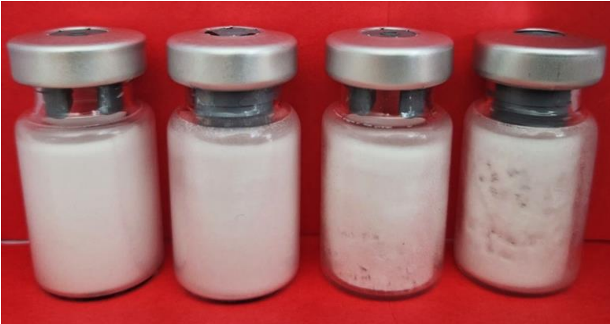
Left to right: unannealed formulation, unannealed placebo, annealed formulation, and annealed placebo
