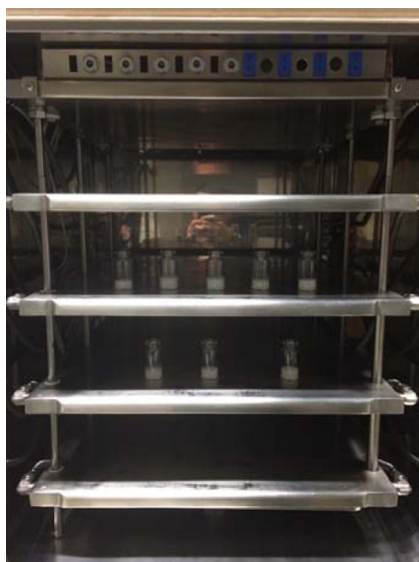
Fig. 1. Lab-scale freeze drying chamber with four temperature controlled shelves.
