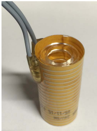
Fig. 2. Spin frozen vial in close contact with surrounding electric heating pad.
