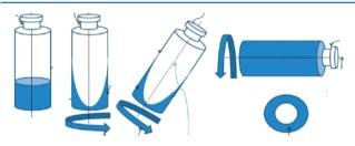
**Figure 1.** Schematic representation of the spin freezing step in a continuous freeze-drying process.<sup>7</sup> Reproduced with permission from ref 7. Copyright Elsevier 2015.
