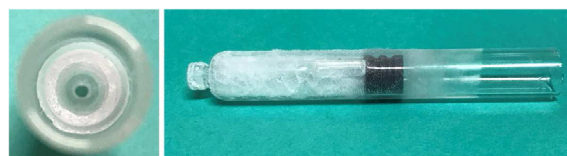
Fig. 5. Visual aspect of the DCC after spin freezing (right) and cross sectional view after removal of the middle plunger (left).
